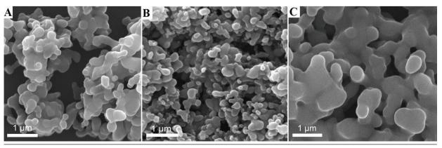
Figure 1: SEM Micrograph of TCP Powders Sintered at A) 1000°C, B) 900°C, and C) 700°C (pH = 7.4)
